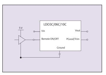
Figure 3 - Remote ON/OFF Input Drive Circuit for Logic Driver
