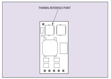
Figure 9 - LDO06C/10C Thermal Reference Point Location Converters
