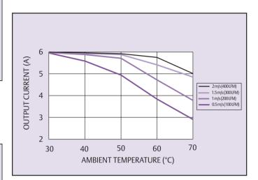
Figure 6 - Maximum Output Current vs. Ambient Temperature and Airflow for LDO06C with Vout Set to 5 V at 12 Vin
