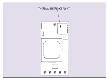
Figure 8 - LDO03C Thermal Reference Point Location Converters
