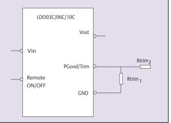
Figure 11 - Output Voltage Trim - with Voltage Source
